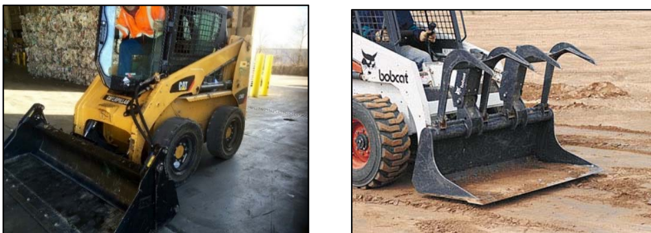
Figure 6: Existing Skid Steer Bucket and Recommended Grapple Attachment
